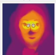
The most reliable area of the face is the corner between the eyes and the nose. In this way, the temperature at the tear ducts is measured
