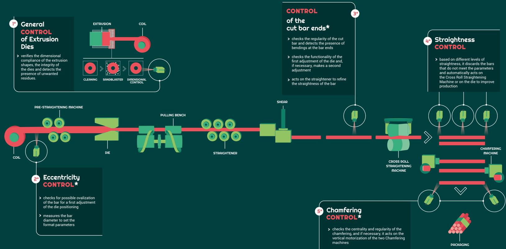
parameters of the various line components, respecting the cycle time. Thanks to the always available production data, it is possible to intervene in real time in case of drifts and repeated errors due to variables on the machinery.
